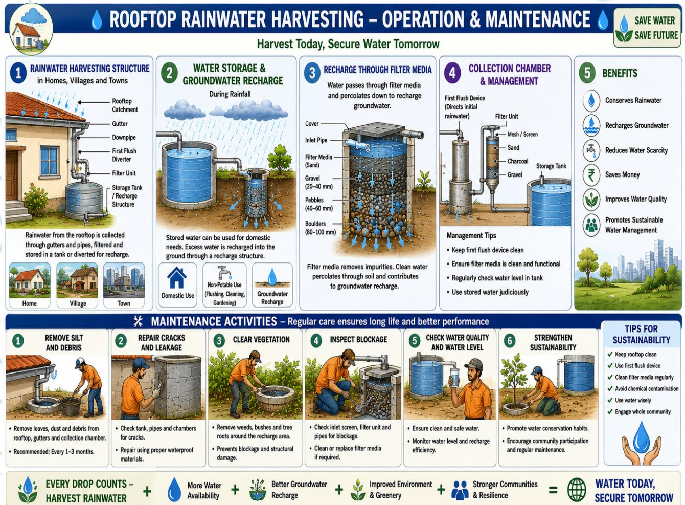
Figure 4: Operation and Maintenance activity for Rooftop Rain Water Harvesting Structures.
