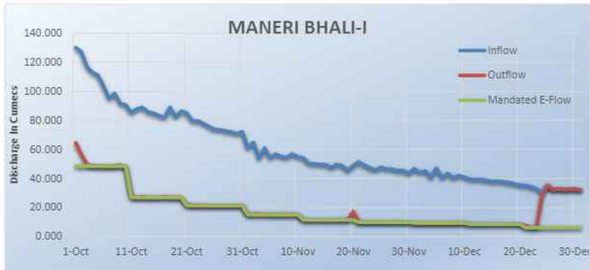
Figure 2: Graph showing status of implementation of e-flows at Maneri Bhali Phase I Project.
